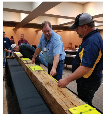
Lawrence Jones and Steve Bryant of Stella-Jones measure the rail-bearing area while Ethan Lightcap of Stella-Jones takes a closer look at the tie.
